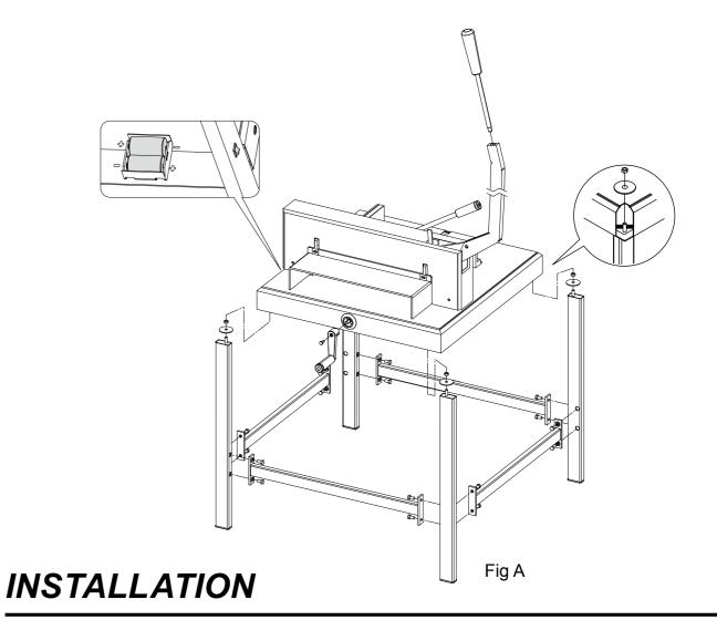
The grip of the knife lever has been careful packed with machine together. Please install these items right away.
