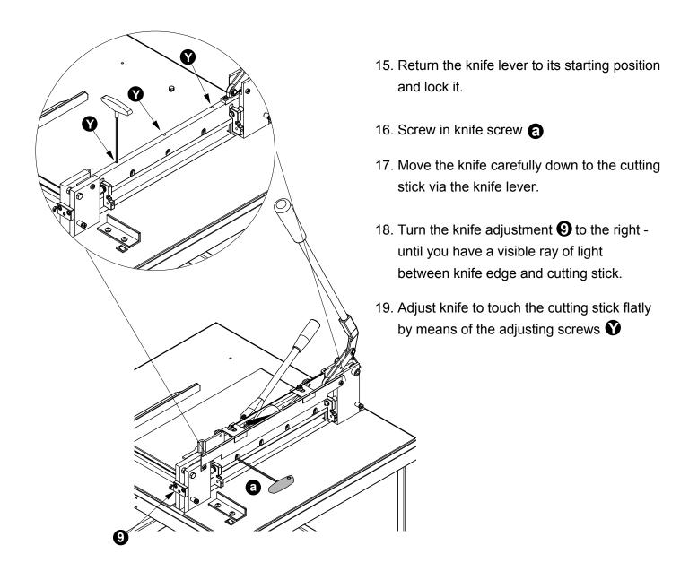
20. Move knife lever to top position and lock it.
